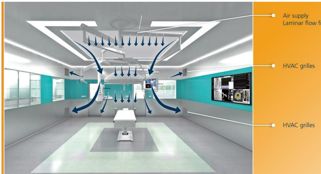
**LAF: Laminar airflow – TAF: Turbulent airflow**
